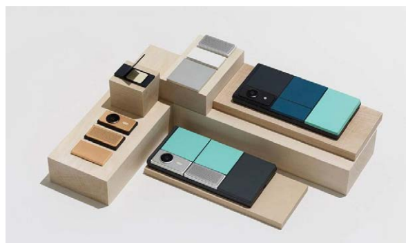
Google's modular smartphone Ara can be built from the frame up by the user, almost like a Lego.
